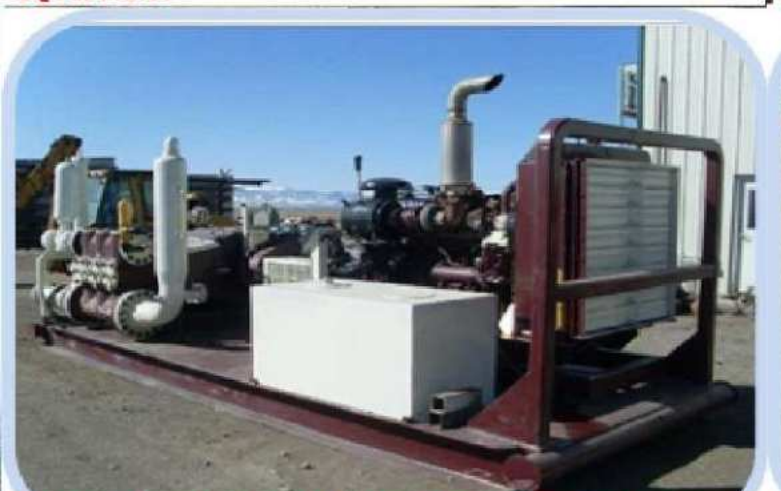
1500PSI TRIPLEX PUMP FOR HYDROBLASTING SERVICES
