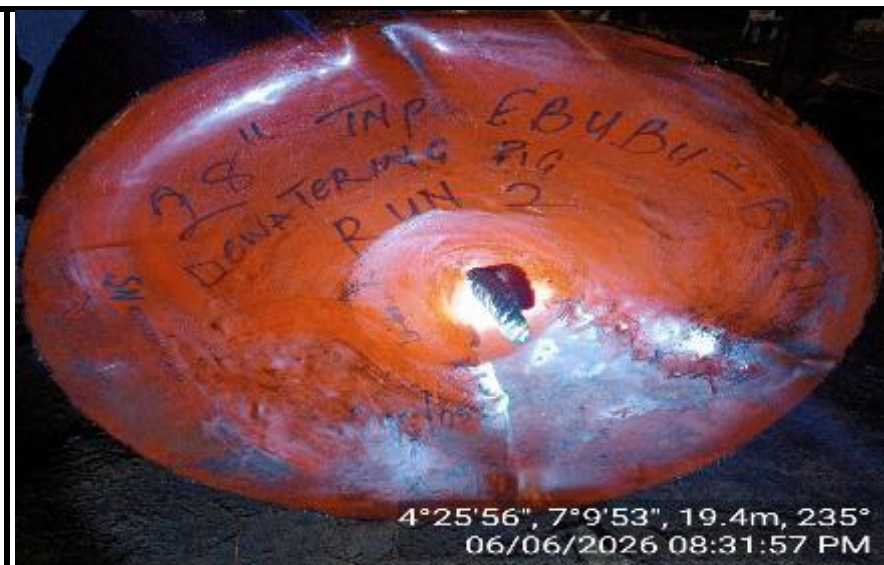
DEWATERING PIG – RUN 2
