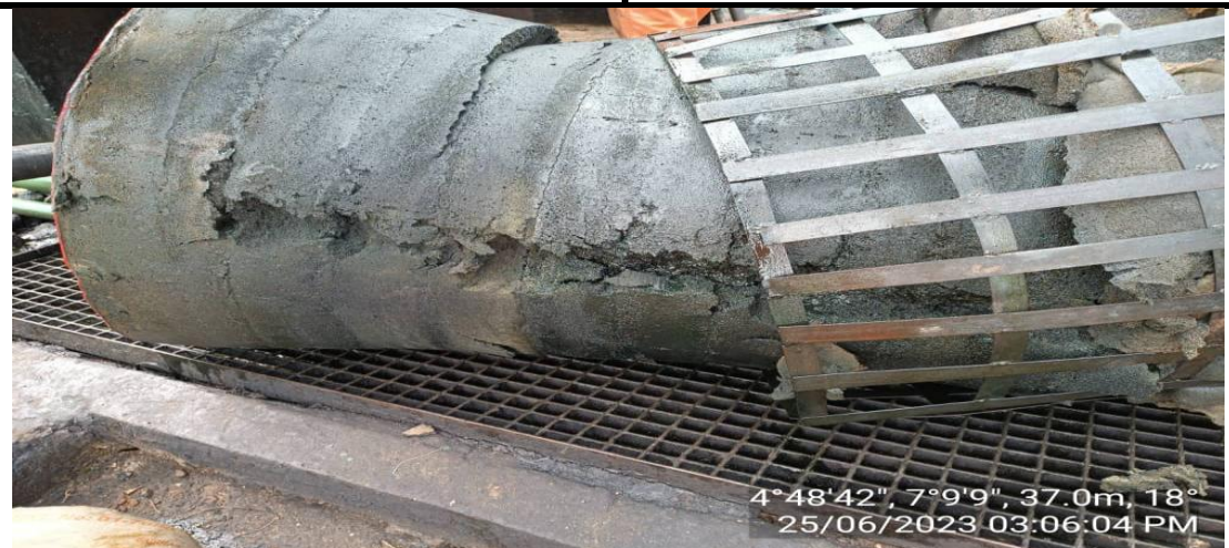
LOADED 36" MD COATED FOAM PIG (RUN 2)
