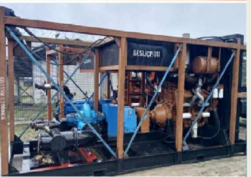
54BBLs/MIN @ 365Psi PIPELINE FLUSHING & FLOODING EQUIPMENT
