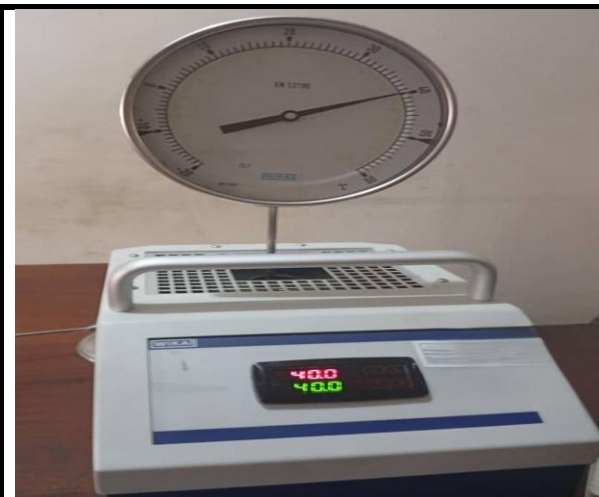
CALIBRATION OF TEMPERATURE GAUGE
