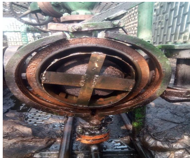
RECOVERING OF BATCHING FOAM PIG
