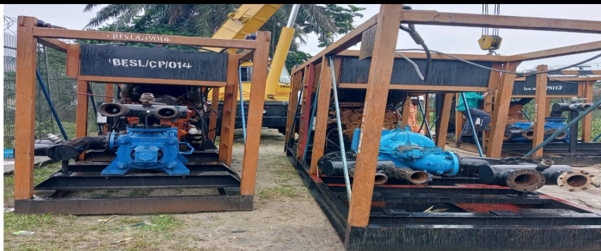
PUMP SPREAD FOR AUXILIARY PUMPING SUPPORT
