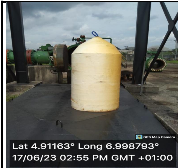
36" MD BARE BODY FOAM PIG READY FOR LOADING
