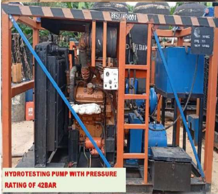
MULTISTAGE(3 STAGE) PUMP FOR FLOODING OF PIPELINE DURING HYDROTESTING
