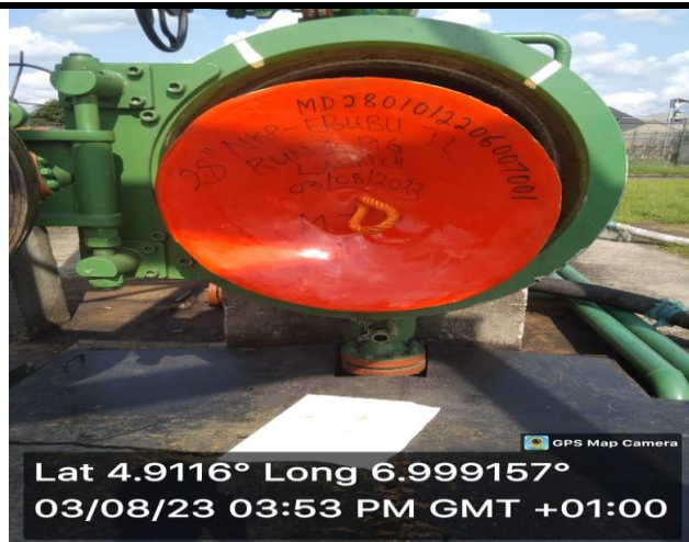
LOADED 28" MD BARE BODY FOAM PIG (RUN 2)
